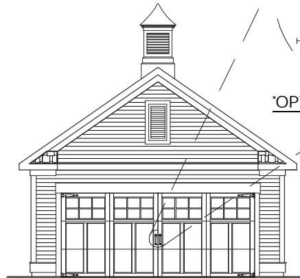
16' x 7' GARAGE DOOR DEL MAR DOUBLE 12 LITE, SQUARE TOP CARRIAGE HOUSE DOOR BY WAYNE DALTON www.waynedalton.com
